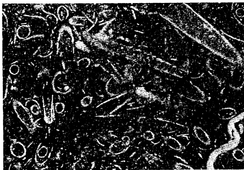
Figure 23. Photomicrograph (plane light) of bioturbated, argillaceous, Styliolina-rich, micritic limestone of Selinsgrove Limestone Member, from cut along Conrail tracks, 1.0 mile northeast of Newton Hamilton. (t=trilobite fragment).
