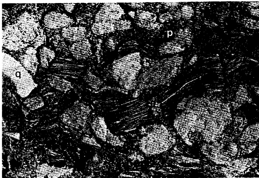
Figure 21. Photomicrograph (plane light) of sandy tuff of Tioga middle coarse zone, from cut along Conrail tracks, 1.0 mile southwest of Newton Hamilton, Mifflin County, Pennsylvania. (f=feldspar, q=quartz, b=biotite, p=pyrite, g=groundmass)
