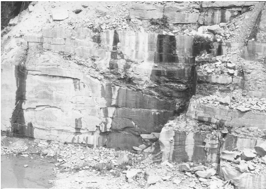
Figure 63. Channel cutout in massive sandstone of upper cycle in new quarry at Site A. Staff is 5 feet long.
