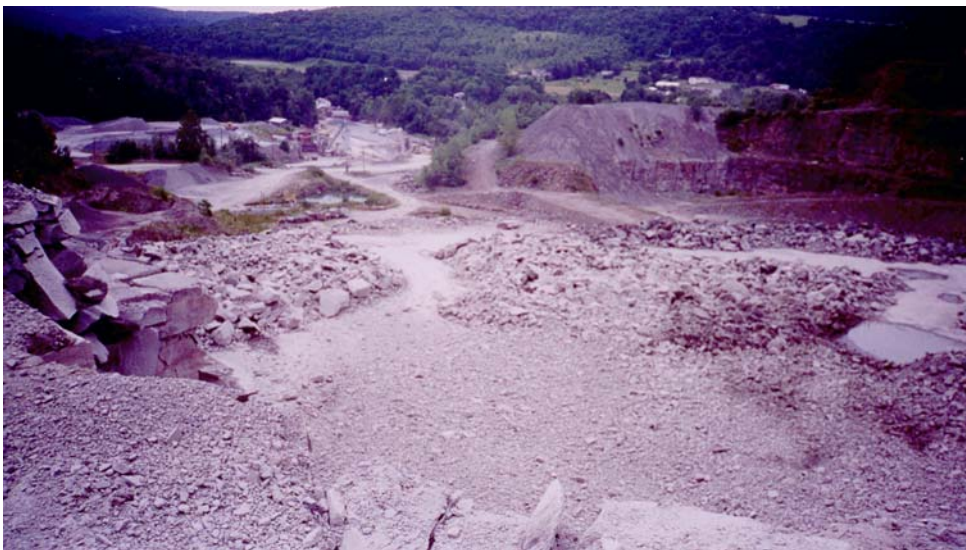
Figure 52. Fragmented rock on Level 1 resulting from blast of July 25, 2002.
