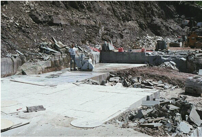
Figure 85. On-site cutting of sandstone blocks for production of "pattern flagging" at the "lower" quarry.
