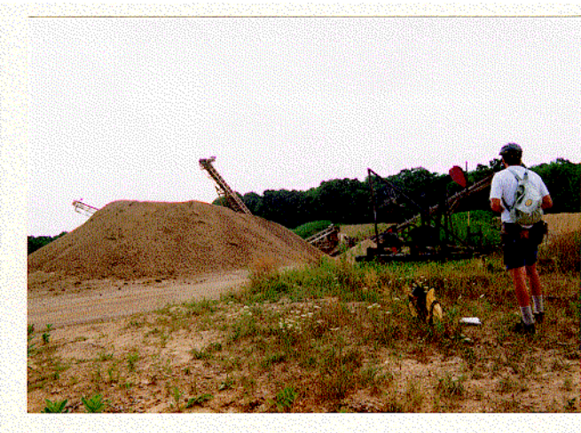
Figure 8. Sand and gravel operation in glacial outwash on the Allegheny River near Franklin, Venango County.
