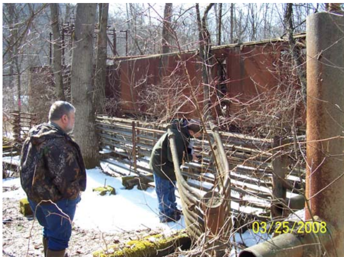
Figure 6. Top—Casinghead gasoline compressor at Columbia Farm. Bottom—Compressor coils.
