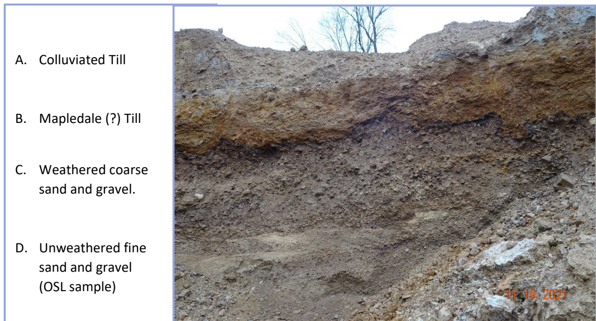
Figure 5.5. Southeastern pit wall, Vincent Pit. Cross bedded sand and gravel lenses at base of pit (D), overlain by dark, cemented sand and gravel (C), and till (B). Colluviated till at top (A). Manganese accumulation in coarse, weathered sand and gravel at the contact with the overlying weathered Mapledale(?) Till. OSL sample 11-29-21 taken in basal unweathered sand.
