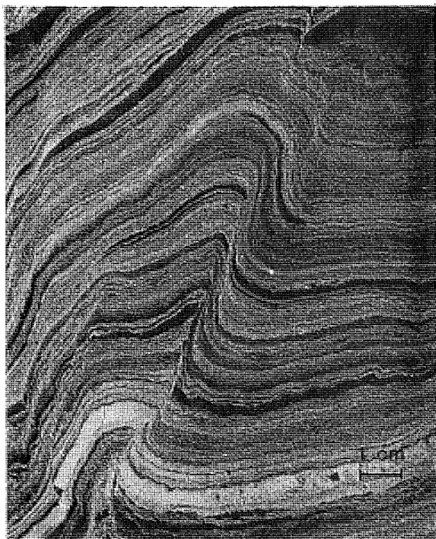
Fig. 105. Negative print of acetate peel stained with alizarin red and potassium ferricyanide showing laminated limestone (dark), calcareous dolomite (medium gray), and dolomite (light gray) in the Poxono Island Formation with cleavage developed in steep limbs of crinkles.
