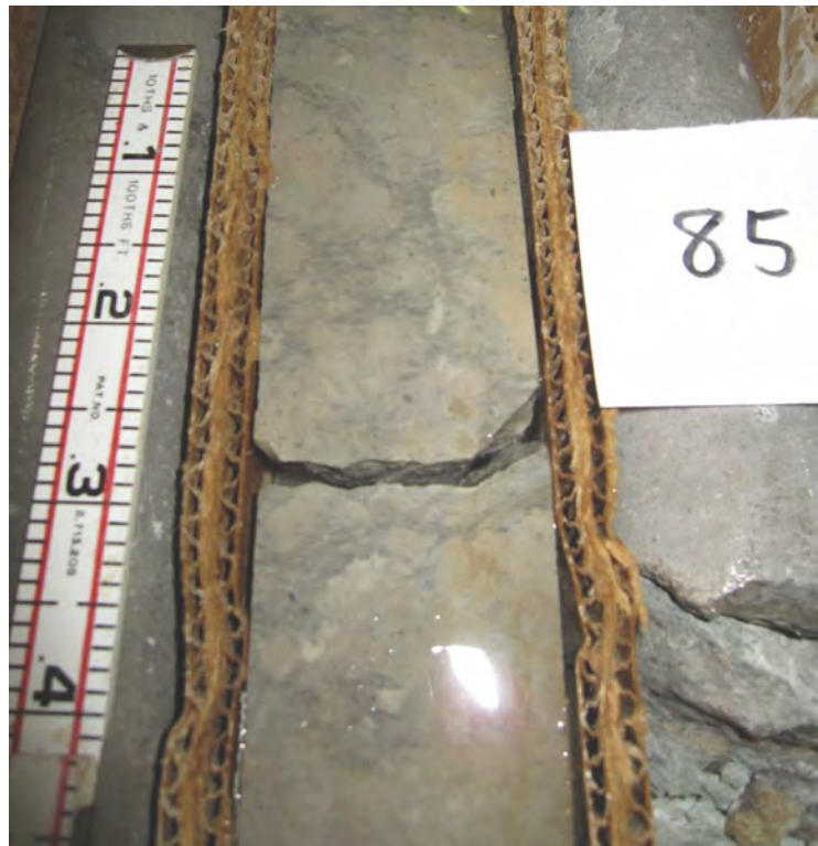
Figure 4 - Photograph of slabbed core from the Gil 30 core at a depth of 85 feet. The limestone is mostly light to medium brownish gray, microgranular, dolomitic, and can range from massive to nodular. Brecciated textures are prevalent.
